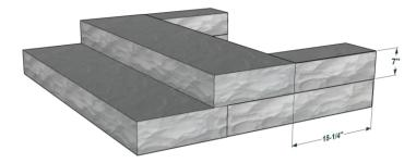
Cut one filler into two equal pieces and place it behind the second step. STEP 3
